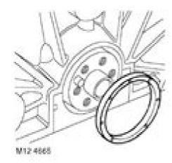
Carefully remove oil seal from cylinder block to avoid damage to seal location or running surface on crankshaft. Discard seal.
