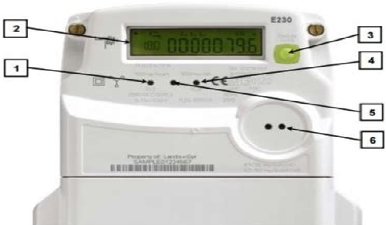
Figure 3. View of the E230 ZxR110CC meter
